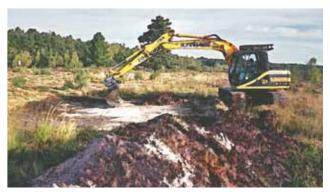
Machinery such as a 13 tonne, tracked, 360° excavator is suitable for creating natterjack scrapes (John Buckley)
